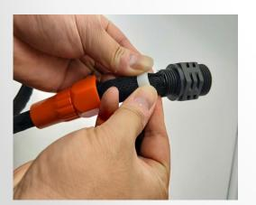
4. Ensure of locking the C-buckle, push the hex joint upward and tighten the water pipe in the right hand.
