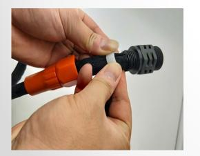
4. Ensure of locking the C-buckle, push the hex joint upward and tighten the water pipe in the right hand.
